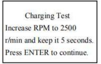
Tester starts the charging volt test after increase rev detected.
